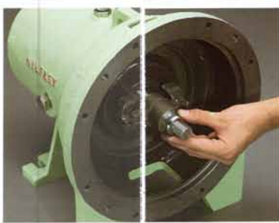
17. Slide expeller O-ring onto the shaft and properly seat it against the governor sleeve assembly.
