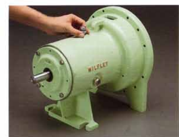
6. Install sight glass, fill plug and drain plug (not shown).
