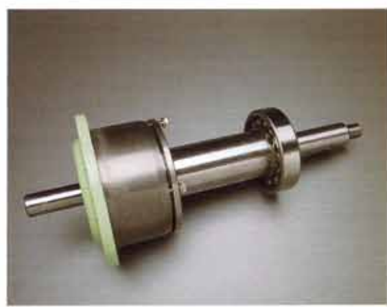
2. With the bearings installed, assemble the rear bearing housing. Be careful not to damage the bearing retainer housing oil seal (not shown).
