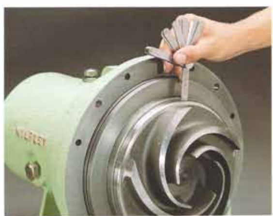
21. Check clearance between impeller and case plate.
