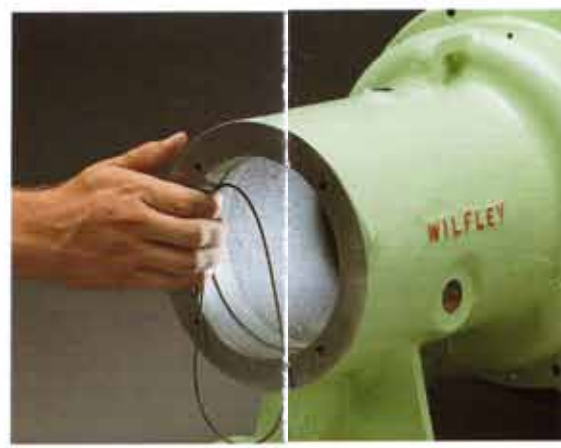
3. Lubricate and install frame O-ring.
