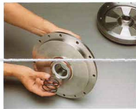
13. Place the governor spring inside the rotary seal housing. Be especially careful not to damage the rotary seal housing seal.
