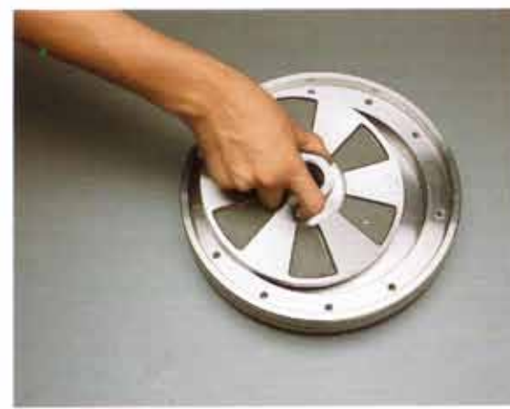
9. Place the expeller (vanes up) into the cavity of the case plate.
