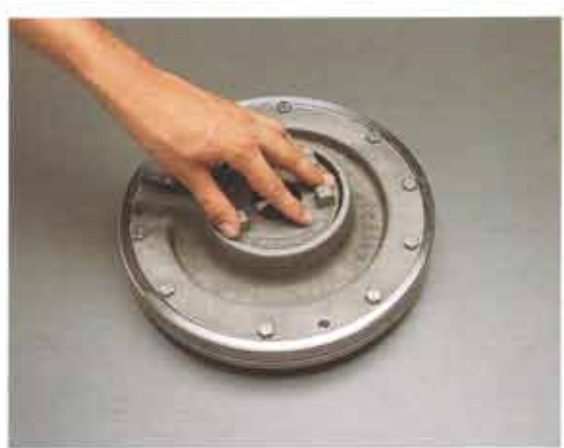
16. Install and tighten stationary seal ring housing cap screws and push down on entire unit to test for the proper action.
