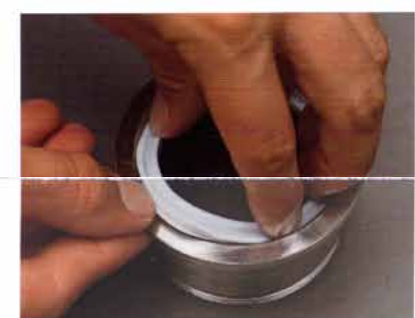
10. Special care must be taken to ensure that the lips of the rotary seal housing seal are not damaged. Install so that the seal seats properly and is not distorted.
