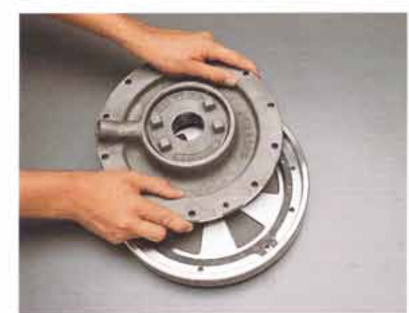
15. Insert the rotary seal housing and stationary seal ring assemblies into the case plate assembly.
