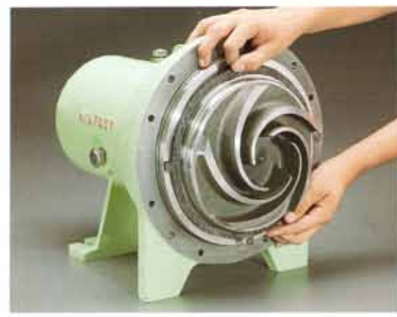
23. Position case gasket on the case plate.
