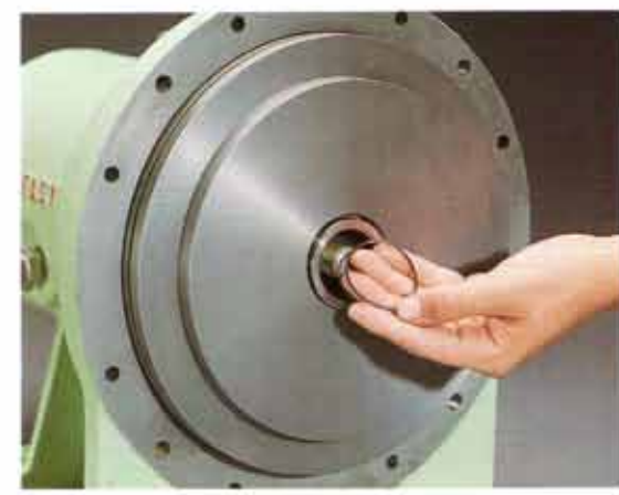
19. Slip the entire case plate assembly over the pump shaft and into the frame cavity and install expeller O-ring.
