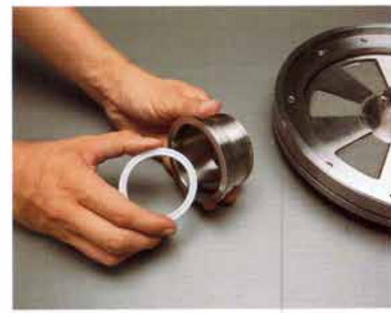
9A. Install the rotary seal housing seal in the rotary seal housing.
