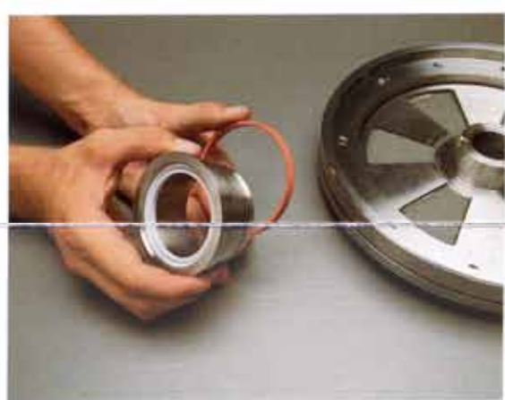
11. Install the rotary seal ring on the rotary seal housing.
