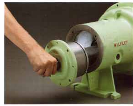
5. Carefully install shaft assembly into frame.
